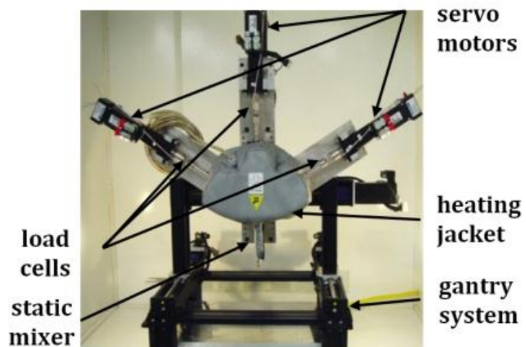
Figure 2.1. The triple-extruder Freeze-form Extrusion Fabrication (FEF) machine.
